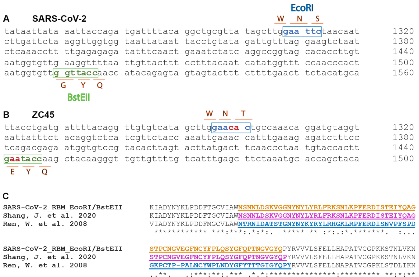
Figure 5. Two restriction sites are present at either end of the RBM of SARS-CoV-2, providing convenience for replacing the RBM within the spike gene. A. Nucleotide sequence of the RBM of SARS-CoV-2 (Wuhan-Hu-1). An EcoRI site is found at the 5'-end of the RBM and a BstEII site at the 3'-end. B. Although these two restriction sites do not exist in the original spike gene of ZC45, they can be conveniently introduced given that the sequence discrepancy is small (2 nucleotides) in either case. C. Amino acid sequence alignment with the RBM region highlighted (color and underscore). The RBM highlighted in orange (top) is what is defined by the EcoRI and BstEII sites in the SARS-CoV-2 (Wuhan-Hu-1) spike. The RBM highlighted in magenta (middle) is the region swapped by Dr. Fang Li and colleagues into a SARS Spike backbone 39 . The RBM highlighted in blue (bottom) is from the Spike protein (RBM: 424-494) of SARS-BJ01 (AY278488.2), which was swapped by the Shi lab into the Spike proteins of different bat coronaviruses replacing the corresponding segments 47 .
